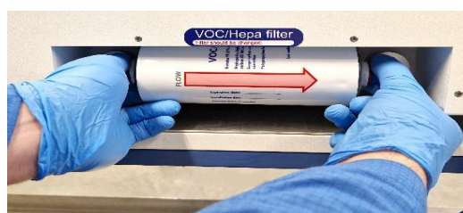
Figure 12.2 VOC/HEPA filter insertion and removal procedure
